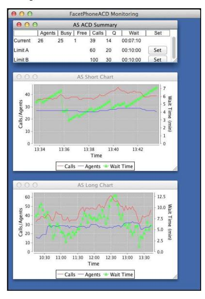
The two graphs at the bottom of the window show the number of calls, number of agents logged in and wait time as lines over time. The top one is on a short time frame to show recent activity close up and the bottom one shows a long term graph of activity.
